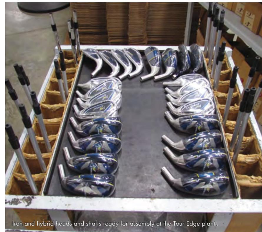
Iron and hybrid heads and shafts ready for assembly at the Tour Edge plant.
